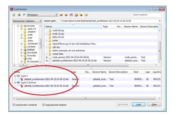
Next, open the Layers tab and select show overlays. Finally you need to check the box next to the layer in order to tell ATLAS what layers to compare.
