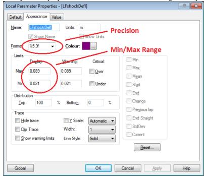
In addition to adding parameters to your waveform, the properties dialog can also be used to format the charts display. Select the display tab to add in a track circuit map, or change the line styles, among other things.
