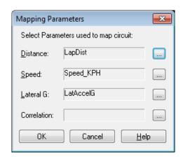
Set the Distance parameter to be LapDistance, the Speed parameter to the function **f\_speedkph** and the Lateral G parameter to the function **f\_lataccelG**, then hit OK. Now go back to the Map tab and adjust the offset until the track looks correct. In addition you may need to select the invert button to give the map the correct orientation.
