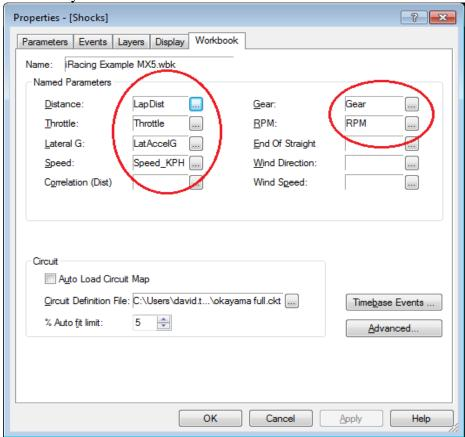
It is especially important that you set up the Distance and Speed parameters. These together let ATLAS display your data in distance mode instead of time mode. Distance mode plots all data against the distance around the race track. This is very useful when comparing data from one run to the next.
