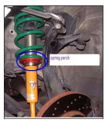
In addition to front ride height and rake, the SPO acts as a camber adjustment for the front wheels. Camber is an important set-up concept because it is used to help maximize the contact patch of the tire during cornering.
